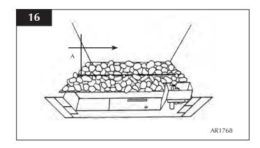
NOTE: IT IS IMPORTANT THE GRANITE CHIPPINGS DO NOT COVER THE PORT AREA IN BETWEEN THE BURNER LEDGES.
